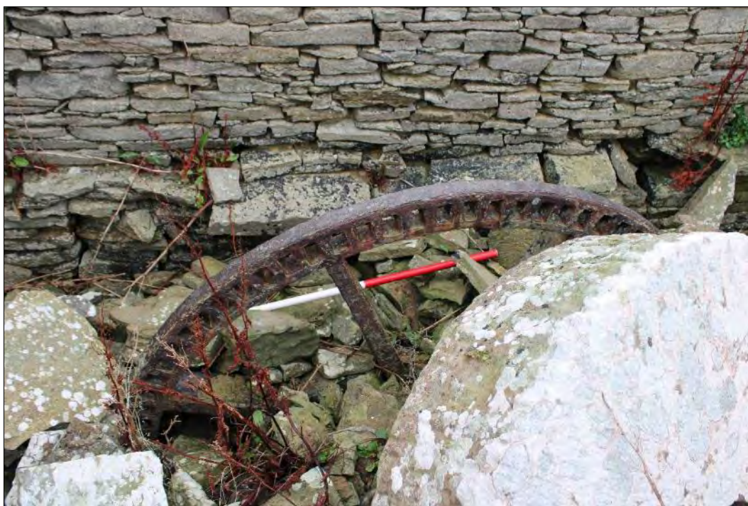
Plate 62: Mill machinery at Hookin Mill. The wheel appears to be in-situ within the demolition rubble and is probably connect to the external mill wheel by a shaft passing through the centre of both.
