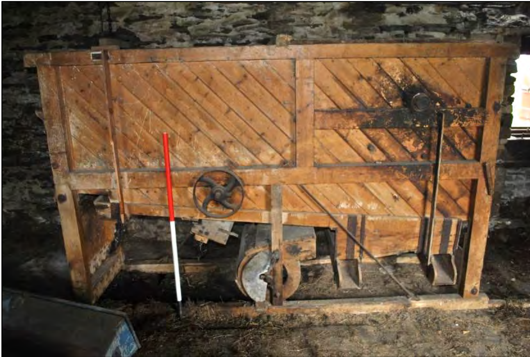
Plate 7: A threshing machine at Quoyfaulds, Eday. These machines separated the grain seed from the stalks and husks. The first threshing machine was invented by Andrew Meikle c.1786 and 300 threshing machines were imported into Orkney between 1850 and 1874. It is probable that the larger farms built or had manufactured, their own bespoke machines. A number of examples survive across the North Isles though they are vulnerable to deterioration through age or neglect.
