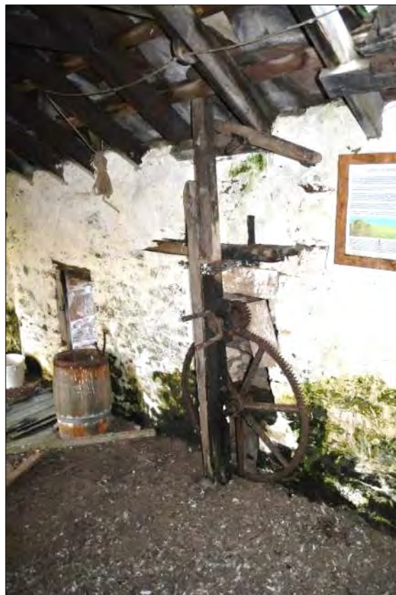
Plate 41: North elevation of Building 17, looking northwest, showing the remains of the mechanism driven by the water wheel. The shaft in the centre of the larger, lower wheel runs through the wall and the centre of the water wheel.
