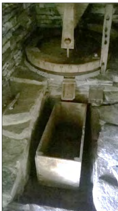
Plate 6: The mill stones inside Click Mill, Dounby concisely illustrate the basic milling process. Grain is placed in the hopper (top centre) and slowly decants through an aperture in the upper millstone of the pair below. These are turned by the water wheel (or mill wheel), with the power transferred by a series of mechanisms and gears. The grain is ground between the mill stones and the flour is expelled into the trough (centre bottom) via the chute protruding from stonework supporting the grindstones. This is the same process seen in the larger mills where the various components would be separated across multiple floor levels.
