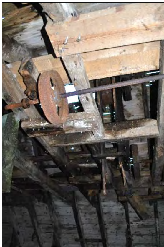
Plate 150: Pulley used for lifting bags of grain from the ground floor to the second floor of the mill building. The pulley is attached to a roof truss and was linked by a mechanism to the water wheel.
